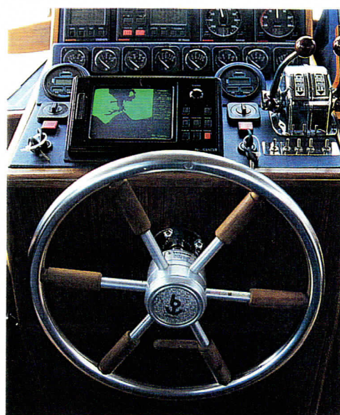
White Mouse II's redesigned helm console, with modern plotter, autopilot and fluxgate compass. Photo by Oli Tennent.
